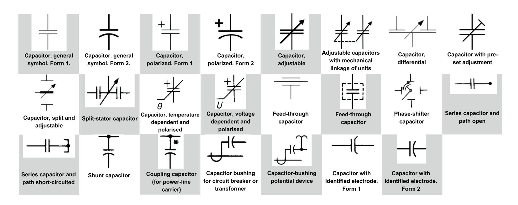
All Electrical & Electronic Symbols in <a href="https://www.asutpp.com">https://www.asutpp.com</a> (based on IEC and IEEE standarts)
