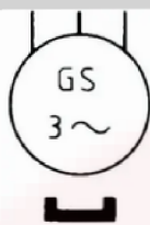
Synchronous generator, 3-phase with permanent magnet
