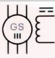
Synchronous generator, 3-phase, both ends of each phase winding brought out
